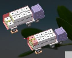
Previously, 18 IBCs were loaded in a 20 ft container. We implemented Maxima IBCs with a reduced height of 5 cm while maintaining the same footprint. These qualified IBCs allow for loading 20 in a 20 ft container, surpassing the earlier design's capacity of 18.
